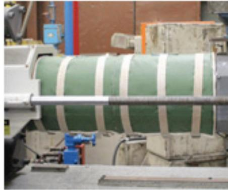
(b) Insulation layer is installed on extruder
