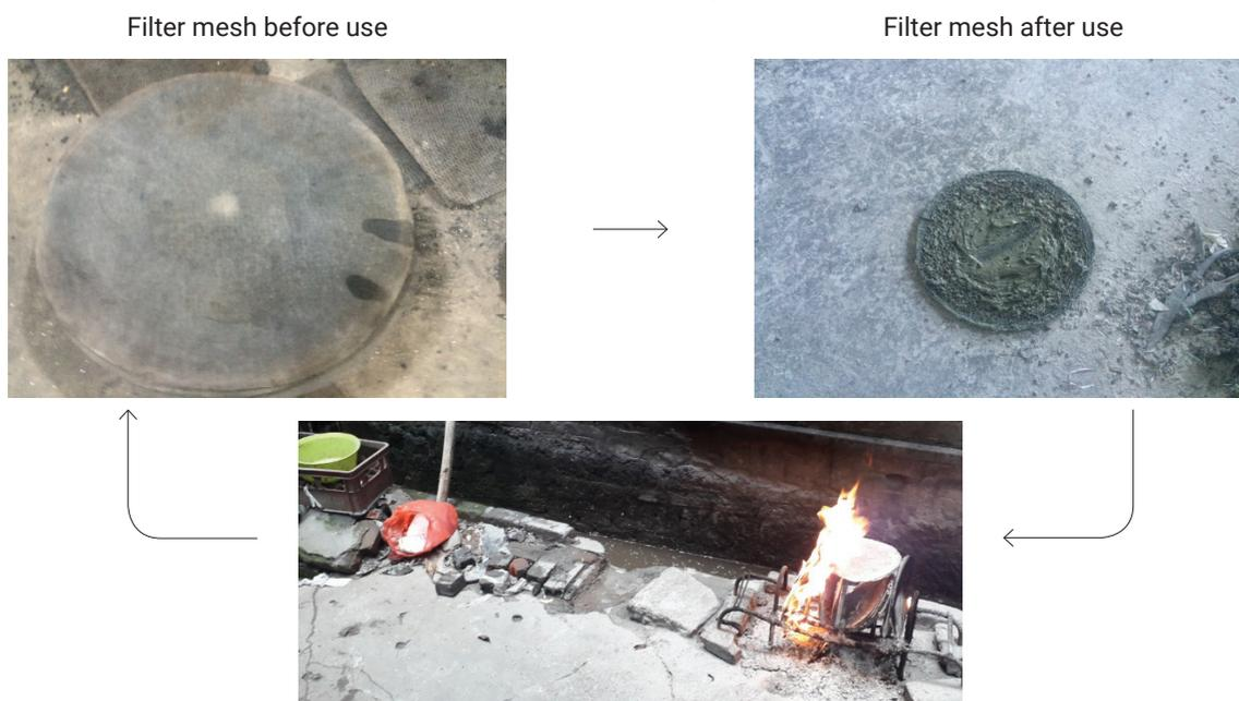
Burning to remove plastics on filter mesh
