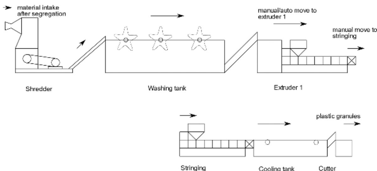
Figure 18. Recycling plastic production by using three-stage wet granulation technology<sup>13</sup>
