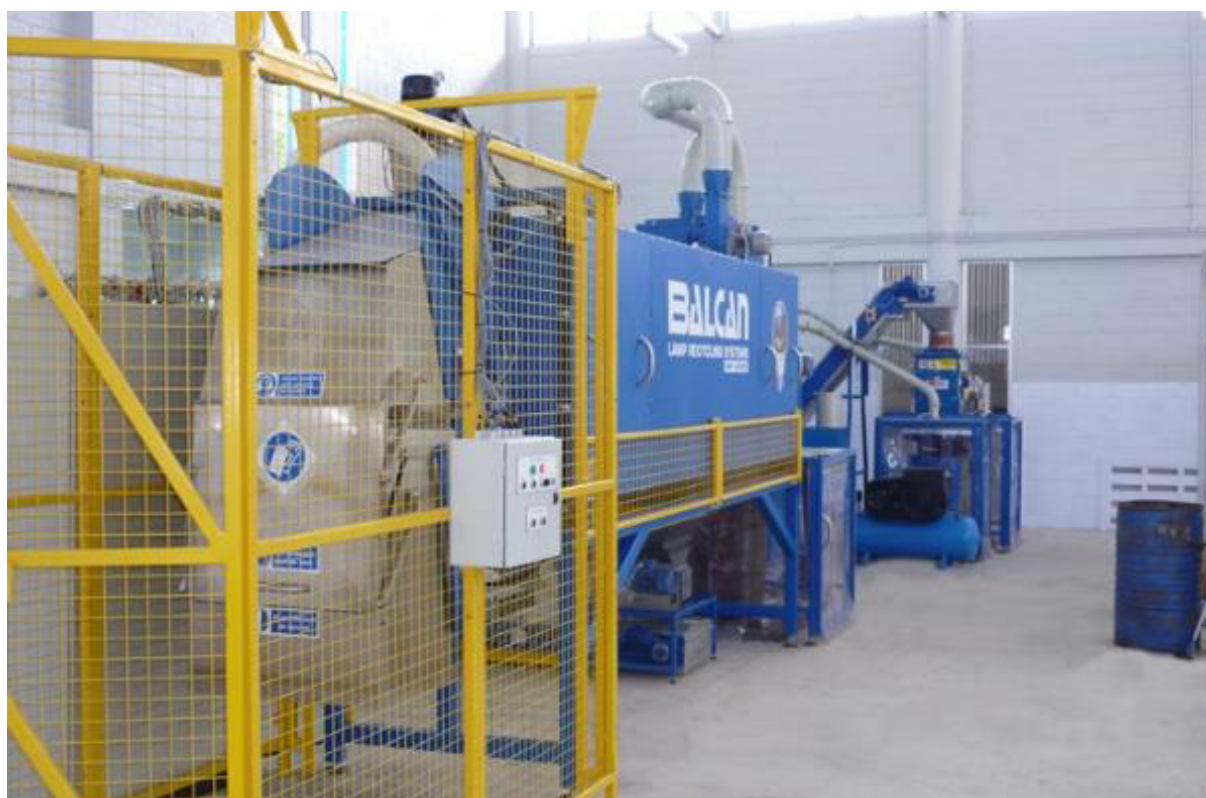
..... Figure 13 A CFL recycling installation at a manufacturer's site in Surabaya, Indonesia, 2013
