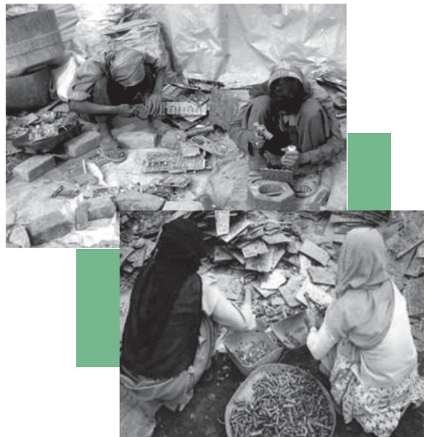
Manual dismantling of Circuit boards
