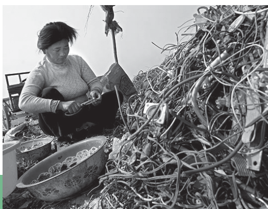
Wire stripping from discarded electronics
